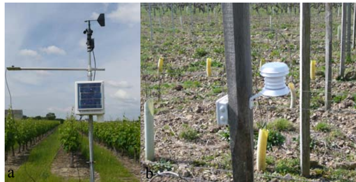
Figure 2. Station Campbell (a) et data logger Tiny Tag (b)
