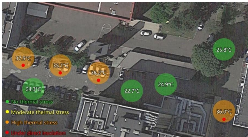
Figure 5. Thermal stress indicator (UTCI) on site before conversion measured on eight different locations on June the 26 th of 2018, from 1 pm to 3 pm (local time)
