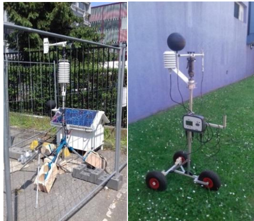
Figure 15: Rooftop (left) and parking lot (center) fixed and mobile (right) weather stations (before conversion).
